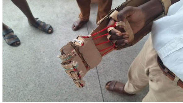
Figure 5: A student demonstrates a bionic arm built from cardboard and strings.
