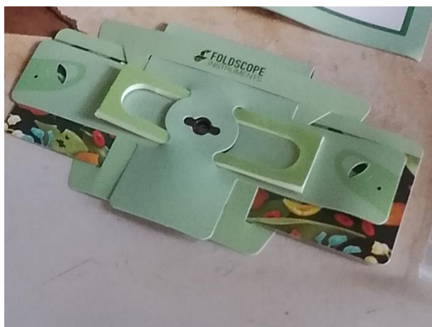
How the foldscope looks once assembled.
